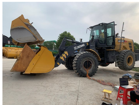
Figure 37. On-site conditions with the rear wheel off the ground.
