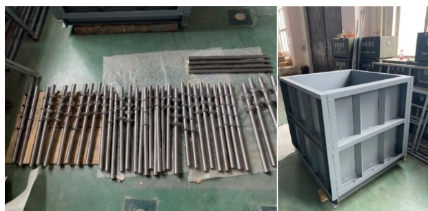
Figure 2. Model pile and box.
