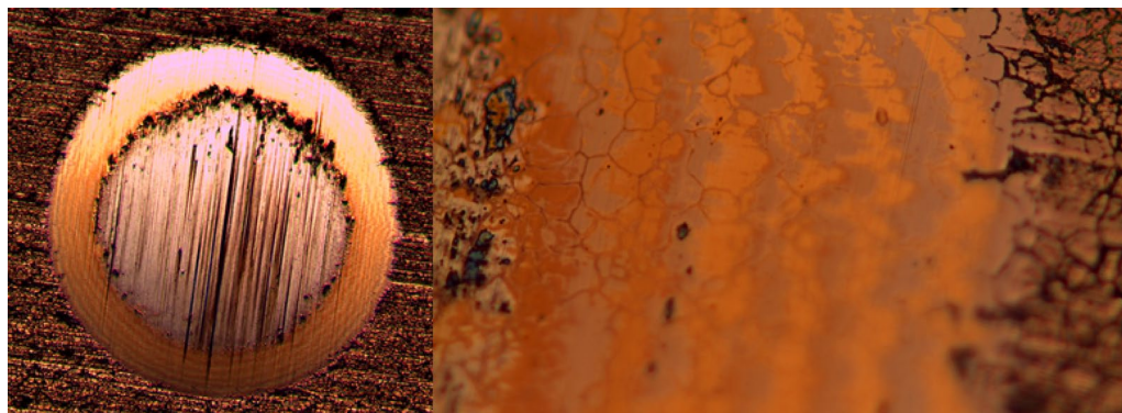
Figure 4. Calotest images for (left image) PN14 at \times 5 and (right image) PN14 at \times 50 .
