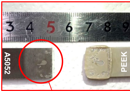
Interface delamination + Partial PEEK cohesive breakdown
