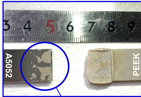
Interfacial delamination + Extensive PEEK cohesive breakdown
