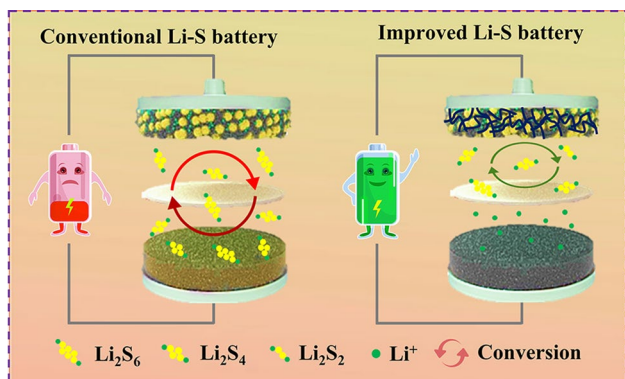
Fig. 5 Schematic of the working principles of Li-S batteries and “shuttle effect” of LiPS
