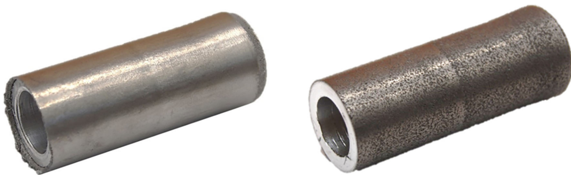
Fig. 19 Cold sprayed Ti coating (25–45 \mu\text{m} , Kinetics 3000, OUT1) on an Al hollow cylinder (left) and the same coating with an additional cold sprayed Al/Ti 30:70 interlayer (45–63 \mu\text{m} ) (right), both after rotary swaging
