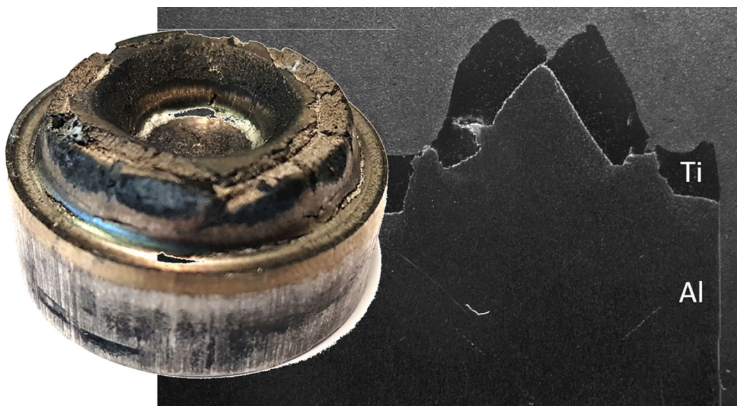
Fig. 15 Al/Ti compound (CS Kinetics 8000-X) die-forged at 350 °C (left) and OM image of the cross-section (right)
