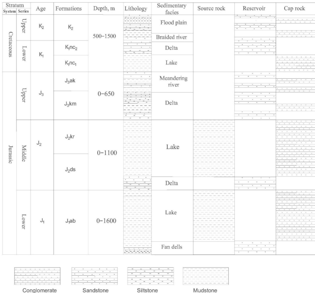
Fig. 4 Schematic section column of the reservoir part of the Arysium depression of the South Turgay Basin, Kazakhstan (Yin et al. 2012)
