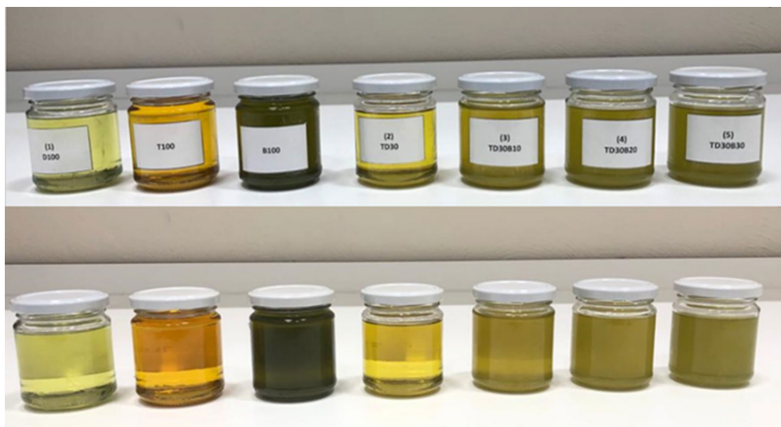
Fig. 2 Waste transformer oil, biodiesel, and euro diesel fuels and blends
